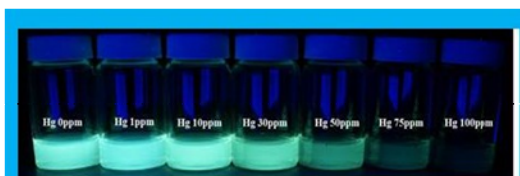
Fluorescence quenching of GQDs with amount of Hg^{2+} ions under 365-nm UV irradiation, showing high removal capacity and high sensitivity toward Hg detection.
